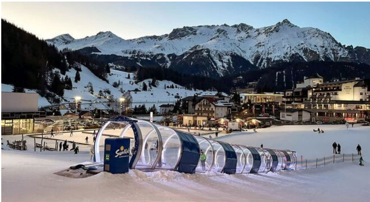
Modern Type N-conveyor belt with illuminated gallery in the “WINTER WUNDER WELT” Nauders, Austria (photo credits: TVB Tiroler Oberland Nauders – Manuel Baldauf)
